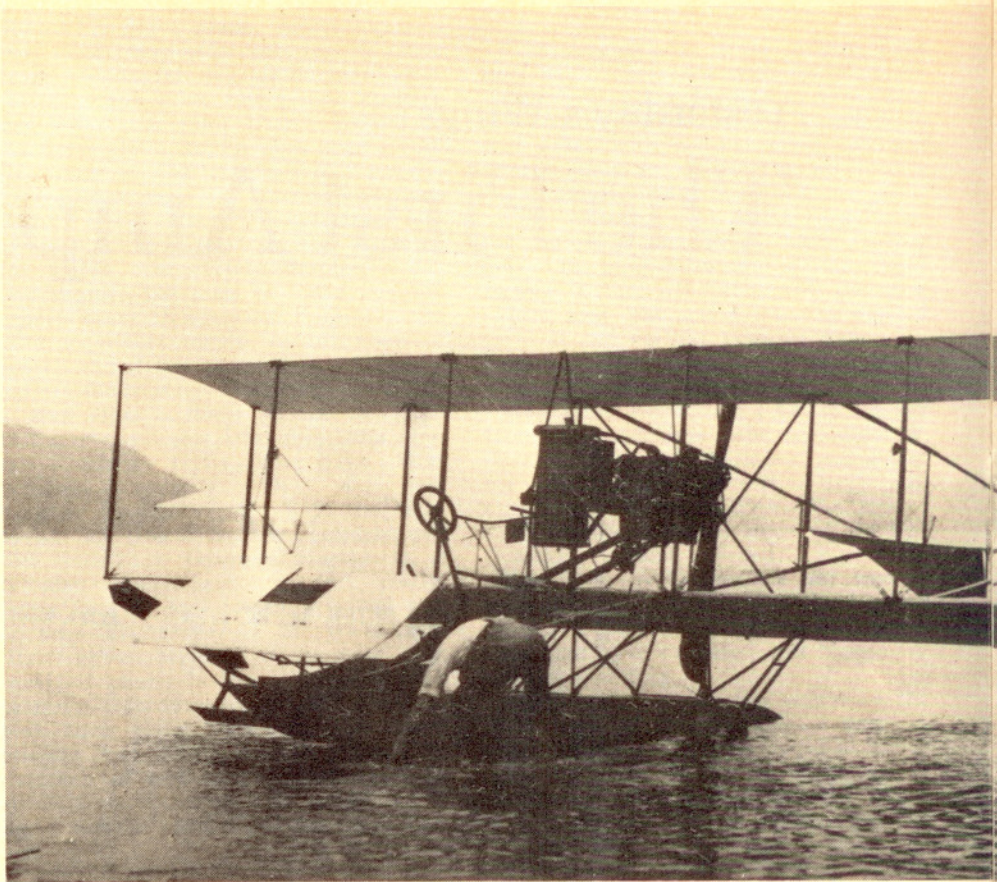
A slightly later Triad on its wheels in shallow water at Hammondsport. Weight has been saved by eliminating the forward booms and attaching the front elevator to the float. Still later Triads and other Curtiss pushers got rid of the forward elevator altogether and were referred to as "headless" pushers.
